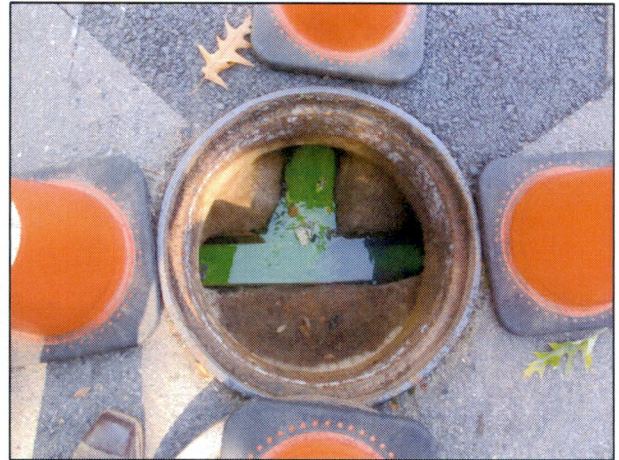
Dye Testing – Topside - Positive (RV13)4075-4073
